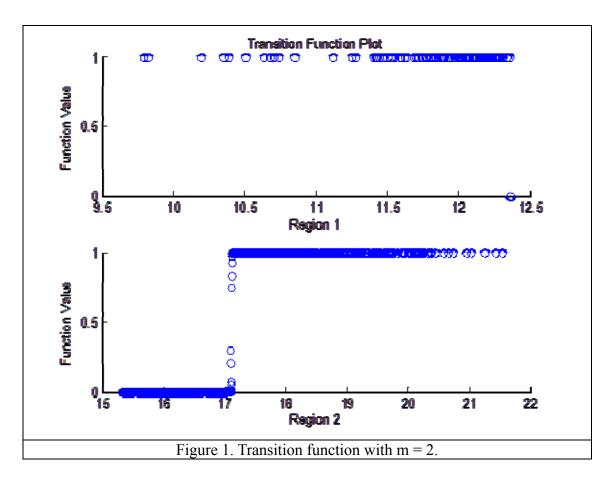
Given the choices of rmax = 3 and m = 2, the optimal (LMF criterion) number of threshold functions is r = 1.
